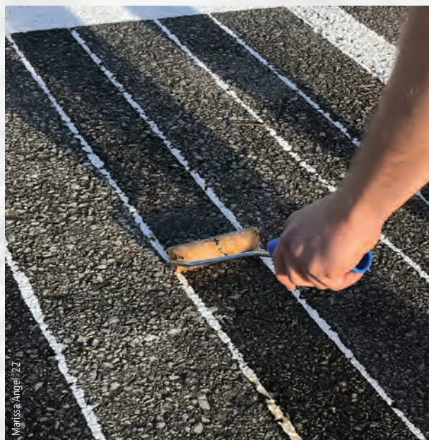
A student uses a soda-soaked roller to test the idea of using Coca-Cola to fracture pavement. Assistant Professor of Design and Sculpture Dan Feinberg teamed up with Dr. Mary Parr, chair of the Agriculture and Natural Resources department, to determine if Coke and radishes could break up pavement and allow for water drainage.
