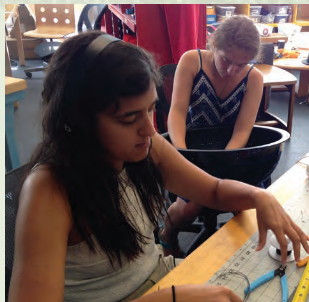
Bianca Godden (left) and Sam Sise (right) installing LEDs into the RTI dome. The reflectance transformation imaging dome allows archaeologists to take better photos in the field without the risk of moving fragile artifacts.
